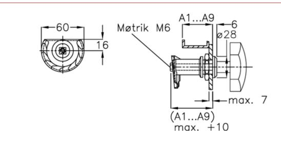
Door + frame thickness = 22-30 Measure type = A2
